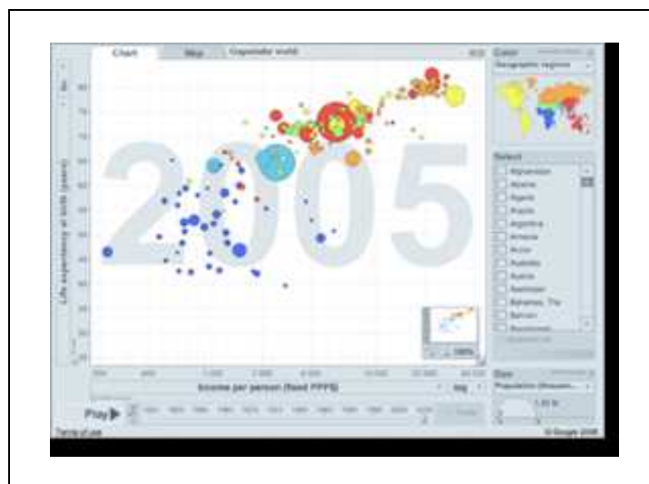
IMAGE 2. Gapminder. Converting time series into moving bubbles, where every bubble is a country.
